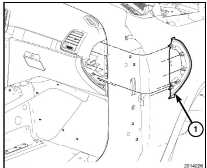
11. Remove the instrument panel center bezel.
