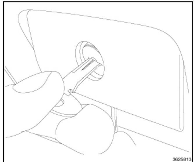
5. Pull the lock cylinder out of the latch.
