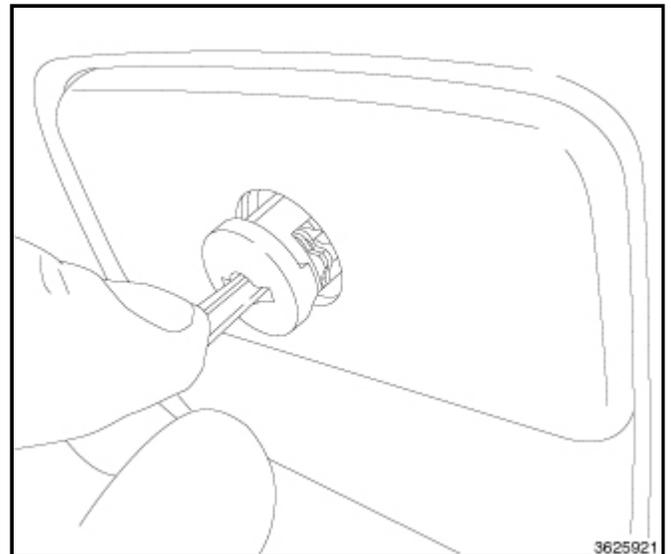
6. Separate the glove box damper (2) from the glove box by sliding the clip towards the rear of the vehicle to release it
