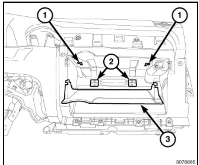
16. Remove the four lower glove box housing screws.
