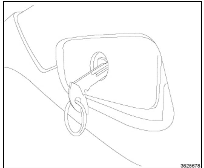
3. Using a small punch or equivalent, push the release tab upward.
