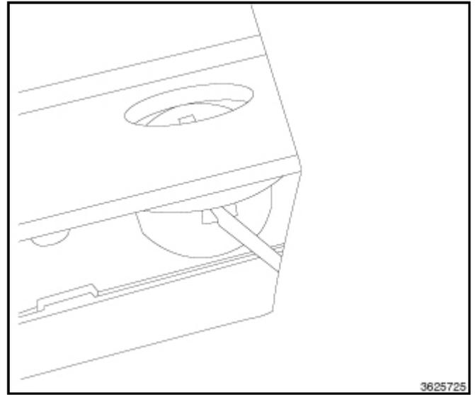
4. Turn the cylinder to the left (counter clockwise). Remove the punch tool and then continue to turn the key to the left until it reaches its full travel and comes to a stop.
