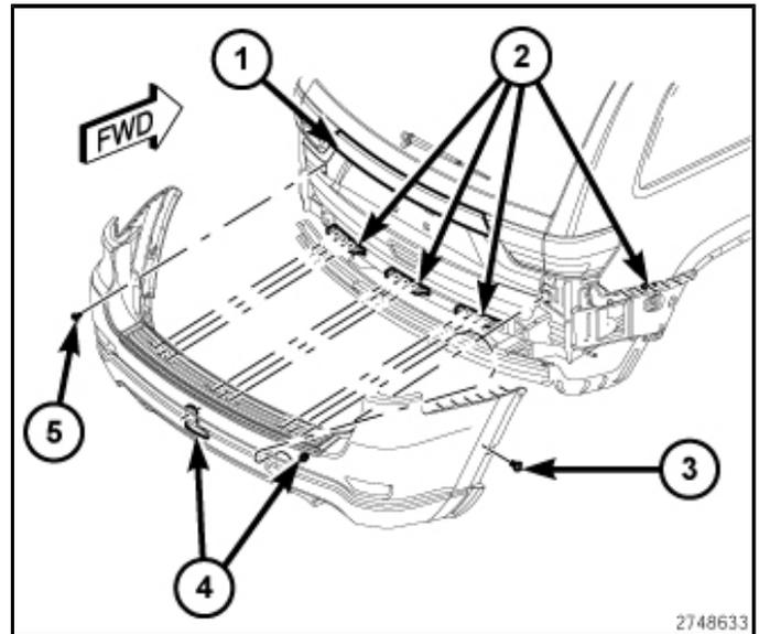
9. Install new rivets (1) at the wheel wells to secure the wheel liners to the rear fascia.
