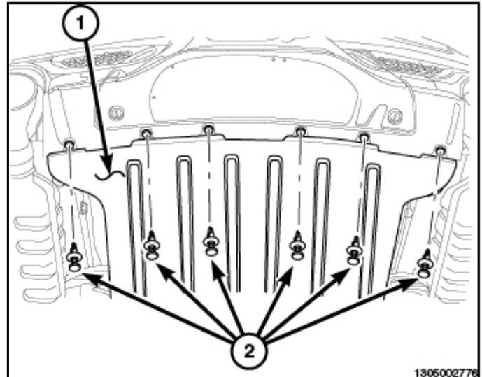
2. Remove the front push pin fasteners (2) and remove the rear belly pan (1).
