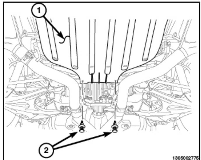
3. Remove the plastic rivets (1) that secure the wheel liners to the rear fascia.
