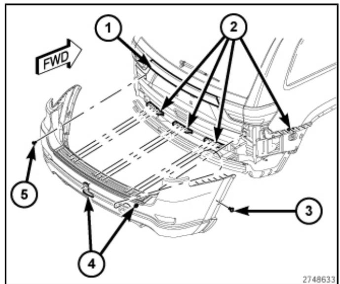
7. Release the integral latch features (2) at the sides and along the back and separate the fascia from the vehicle.
