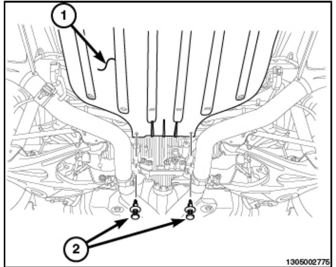
11. Install the rear push pin fasteners (2) securing the rear belly pan (1) to the fascia.
