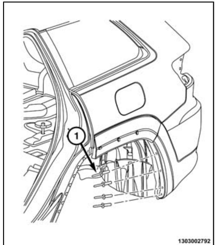
10. Install the rear belly pan (1) and install the front push pin fasteners (2).
