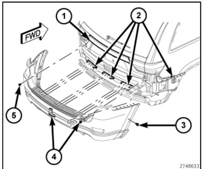
9. Release the integral latch features (2) at the sides and along the back and separate the fascia from the vehicle.
