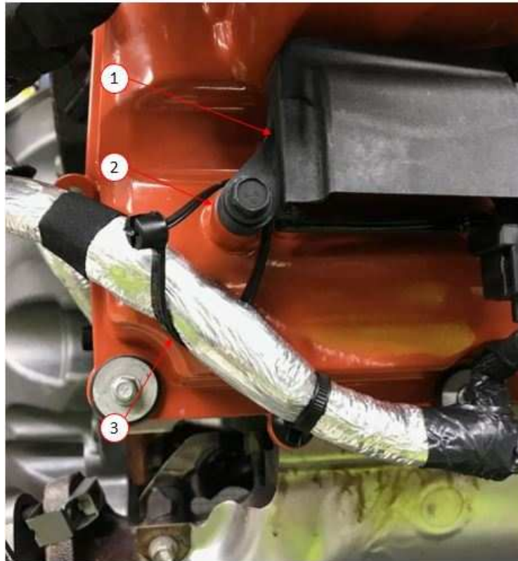
Fig. 3 Location of New Nylon Zip Tie
